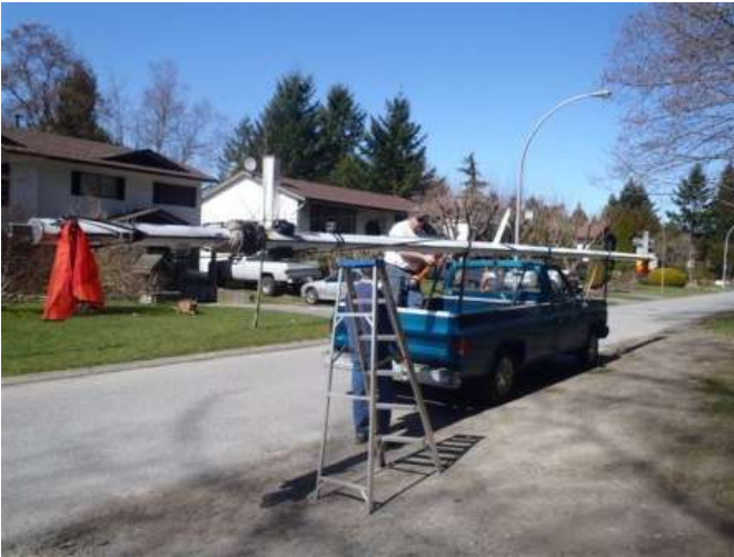
Updated mast fittings, added reacher connection points, new mast step.
